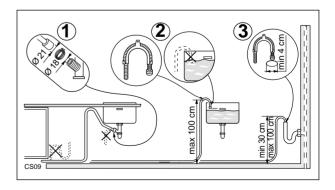
If you use a drain hose extension it must be no longer than 2 metres and its internal diameter must be no smaller than the diameter of the hose provided.
